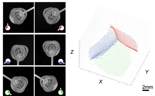
Figure 4. Processed images obtained by the three cameras (left) and the reconstructed leaflet images (right)
