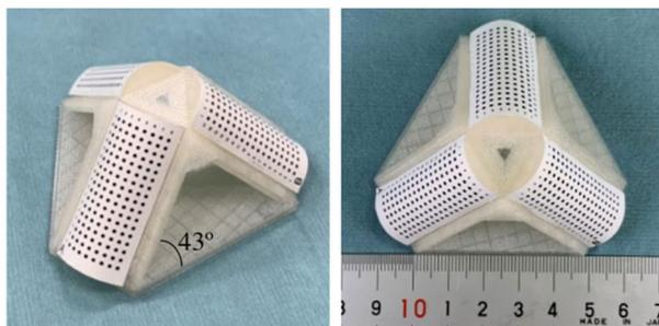
Figure 3. A tetrahedral pyramid-shaped calibrator for the coordinate calibration for the high-speed multi-camera system designed in the study; from the top (left) and the isometric view (right).
