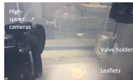
Fig. 1 The multi cameras and the pediatric ePTFE valve leaflet model in the water reservoir used in the in vitro study.
